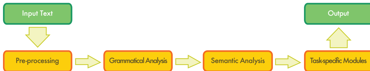
2: A typical text processing architecture
